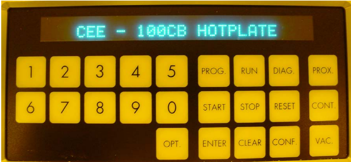
Figure 2. View of the keypad showing the “RESET” and the “PROG” keys. The “OPT” key toggles between the spinner and the hotplate function. This figure shows the “Home” position for the hotplate. This is reached by hitting the “RESET” key and toggling the “OPT” key until this screen appears.
