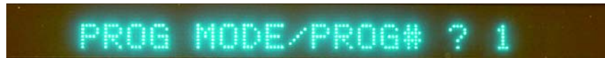
Figure 3. After hitting the “PROG” key, the screen looks like this. It is asking for you to hit a number key to label a new program or call up a previous program.
