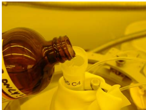
Figure 36. Pouring resist into the syringe. Note the rag to catch spills.
