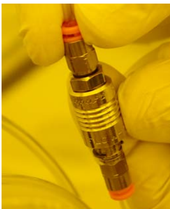
Figure 39. Open the N 2 valve by sliding the sleeve towards the syringe.
