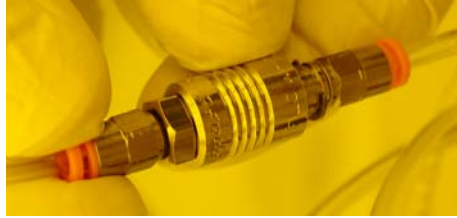
Figure 51. Remember to close the in-line N 2 valve to prevent accidents. NOTE: After you finish your coating operation, clean up all the resist in the spin bowl. Please do this in the solvent hood. Also clean up the hood.
