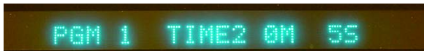
Figure 1. Example of hotplate readout format: Program #1, “PGM 1”; Operation time for step 2, “TIME2”; Number of minutes, “0M”; and Number of seconds, “5S”. Other formats are more self explanatory.
