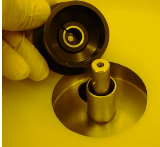
Figure 41. Note the slot in the silver liner in the black chuck and the post on the side of the motor shaft. They must match and seat when attached.
