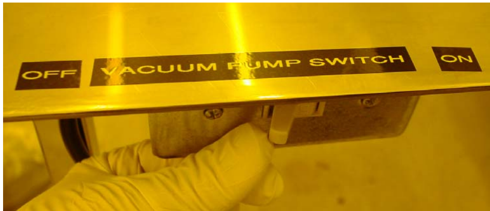
Figure 11. Vacuum pump switch under the right front corner of the table.
