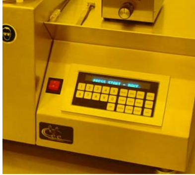
Figure 27. Computer keyboard and readout: Red “On” switch on left of keyboard, “Opt” button at left end of lower key row.
