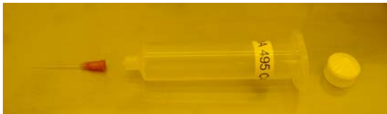
Figure 30. Syringe and needle system. Tip attachment and (white) plug cap.
