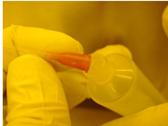
Figure 30. Syringe and needle system. Tip attachment and (white) plug cap.
