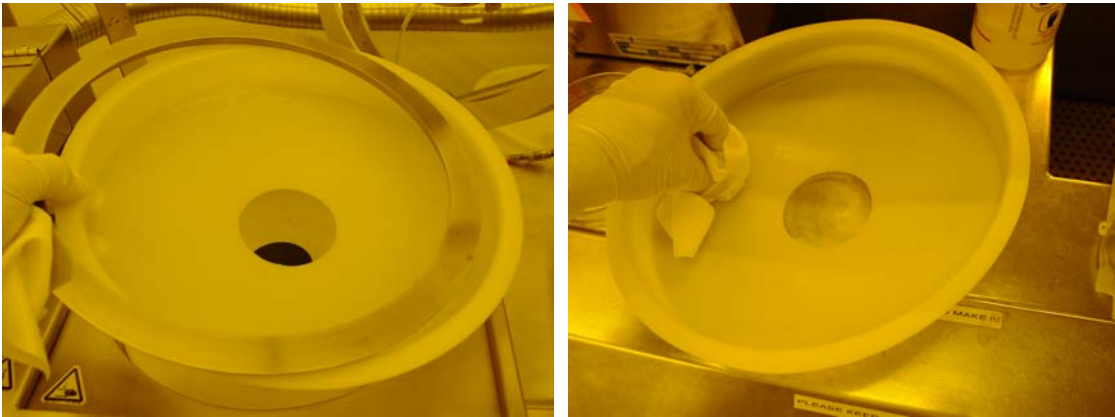
Figure 52. Remove the resist catch-bowl. It just lifts up and the Stainless ring comes right off. Clean it up in the solvent hood with proper solvent for the resist and reinstall it back onto the CEE spinner. (Generally, Acetone will work for most resists.)
