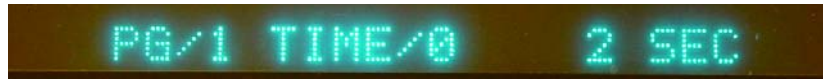
Figure 19. Enter dispense time. Two seconds in the case of low viscosity (watery) PMMA 495 MW C4 E-Beam Resist. The N2 pressure on the syringe is about 9 psi.
