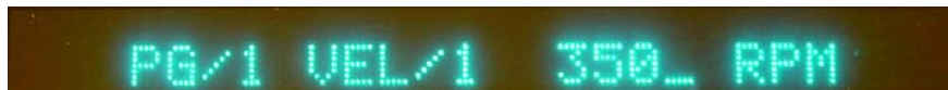
Figure 20. This display indicates that for spin program one, the first velocity is 3500 rpm. (A “0” will appear in the underline position when you hit “0” again.)
