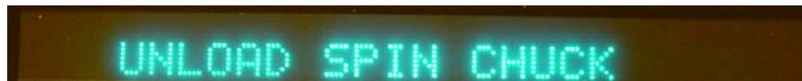
Figure 49. As the wafer is spinning, the display shows the real time spin speed and the time remaining for the spin cycle. At completion, the controller beeps and displays the instructions to remove the wafer. To stop the beeping, hit “STOP.”
