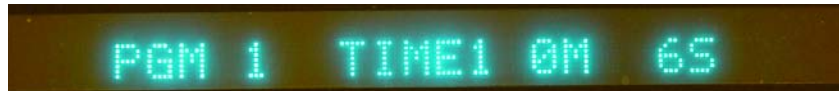
Figure 6. Enter the time in minutes and seconds for the wafer to sit on the gas cushion. Remember to hit enter each time you input a number for the program to go on.
