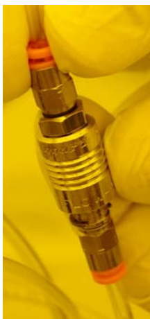
Figure 46. Open the N 2 valve before starting the dispense process... This is easy to forget, but remember, I told you so right here!!!
