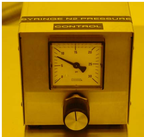
Figure 45. Syringe pressure control. For low viscosity material, use low pressure, for thick viscous fluids, raise the pressure. This constant pressure provides the push to dispense the fluid.
