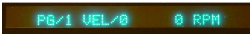
Figure 12. Example readout format: Program #1, “PG/1”; input description Velocity, “VEL”; Step 0, “/0”, and value “0” with units “RPM”. There are other formats that are more self descriptive and will be explained as they are encountered in this paper.
