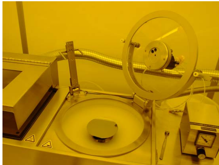
Figure 50. At completion, remove the wafer and close the lid.
