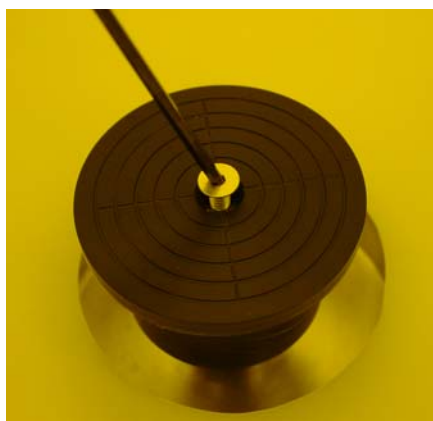
Figure 40. Removing the vented screw to replace the spinner chuck.
