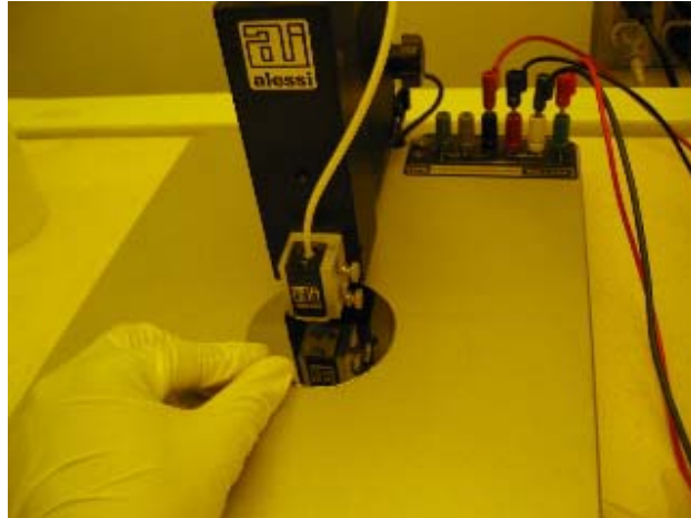
Figure 7 – Place wafer under probe
