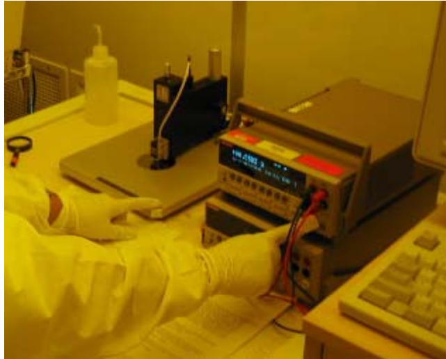
Figure 9 – Measure resistance of the sample
