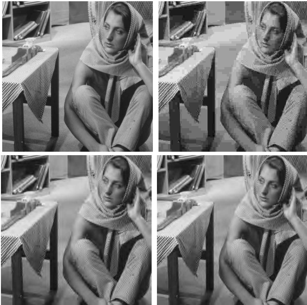
Figure 1.11 Compression of the 512 \times 512 Barbara test image at 0.25 bits per pixel. Top left: original image. Top right: baseline JPEG, PSNR = 24.4 dB. Bottom left: baseline wavelet transform coder [58], PSNR = 26.6 dB. Bottom right: Said and Pearlman zerotree coder, PSNR = 27.6 dB.
