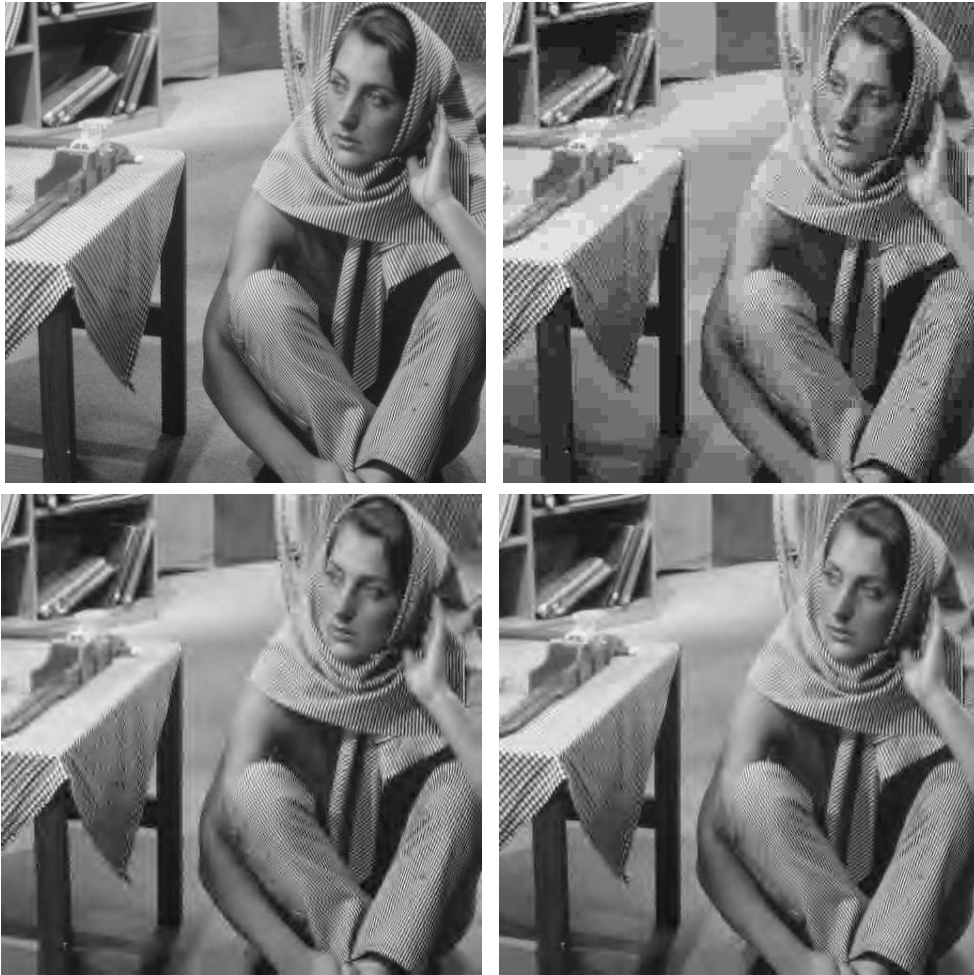
FIGURE 5.16. Results of different compression schemes for the 512 \times 512 Barbara test image at 0.25 bits per pixel. Top left: original image. Top right: baseline JPEG, PSNR = 24.4 dB. Bottom left: baseline wavelet transform coder [19], PSNR = 26.6 dB. Bottom right: Said and Pearlman zerotree coder, PSNR = 27.6 dB.
