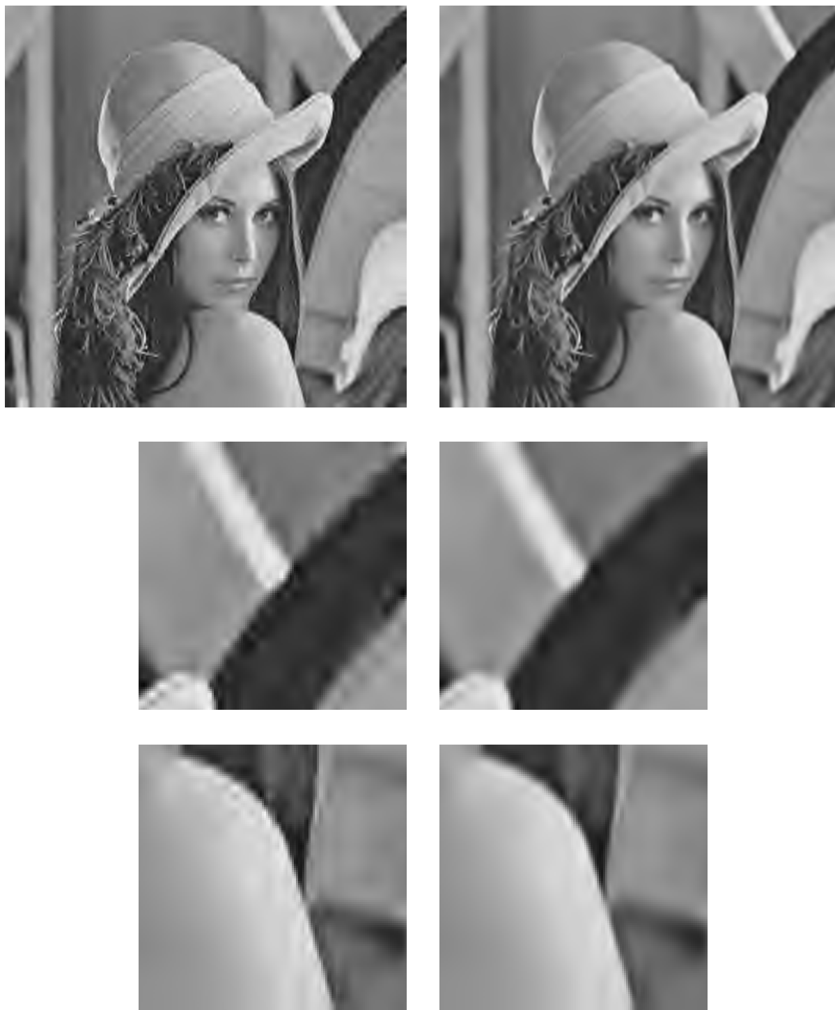
Fig. 4. Compressed Lenna image (left) and post-processed version (right). The magnified portions demonstrate reduction in ringing artifacts.
