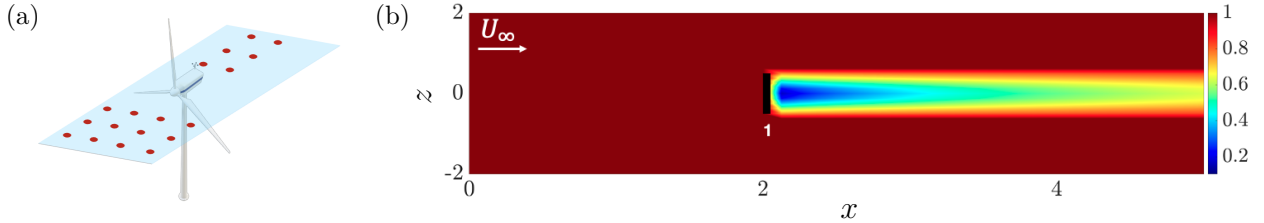
Figure 5.2: (a) Schematic of hub-height computational plane with data points used for training in Section 5.5.1 highlighted in red; (b) Hub-height streamwise velocity \bar{\mathbf{u}}(x, z) generated using the analytical wake-expansion model of Bastankhah and Porté-Agel [8] around which we linearize the NS equations.
