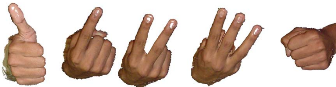
Fig. 4. Static Hand Gestures. From left: “OK”, “One”, “Two”, “Three”, “Zero”. The image is output of the hand localization algorithm.
