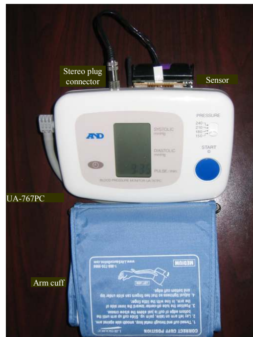
Figure 7. Sensor node interfaced to an A&D UA-767PC BPM.
