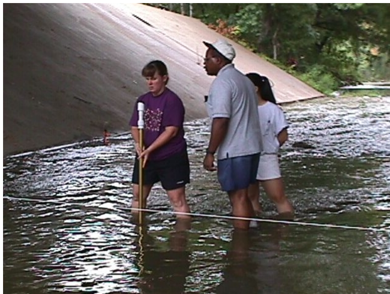
Figure 2.7: Students using an impeller flowmeter. Streamflow from left to right.
