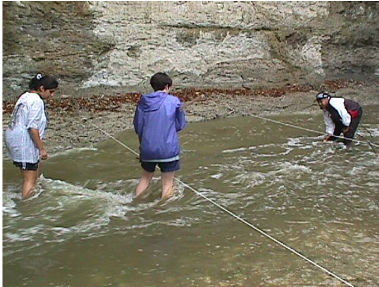
Figure 2.5: Students using the float method for velocity measurement (click on image for full-sized version). Fall '98 class, at Spring Creek, Richardson, Texas.
