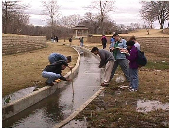
Figure 2.2: Students gauging Cottonwood Creek, UTD. Taglines are used to provide reference elevation, yardsticks or gauging staff are used to measure distance to water and streambed from the tagline.
