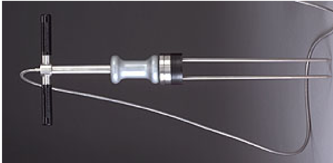
Figure 9: Time-domain reflectometry probe. Signal propagates down probes, reflects from end, travel time is measured at top unit. See SoilMoisture, Inc. and TDR animation.
