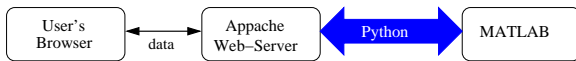
Figure 3. Communication mechanism used in the implementation of the web-based interface for the STP state model.
