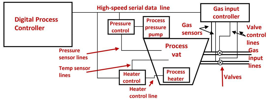
Block Diagram, Process Control System
