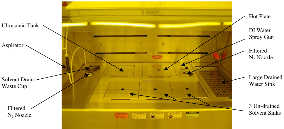
Figure 1. Photo of 6' General solvent hood showing the layout of components on the work surface.
