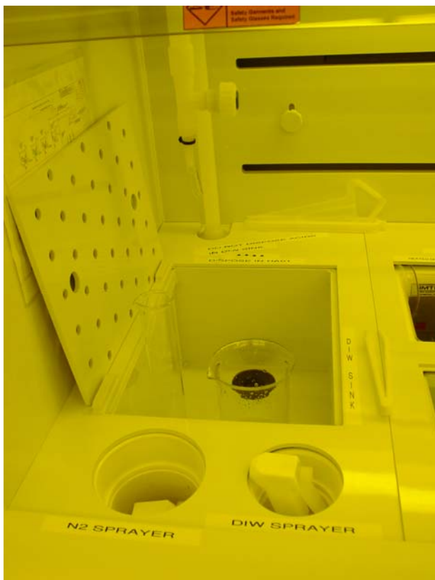
Figure 5. This DI water sink cannot accept waste acids for neutralization.
