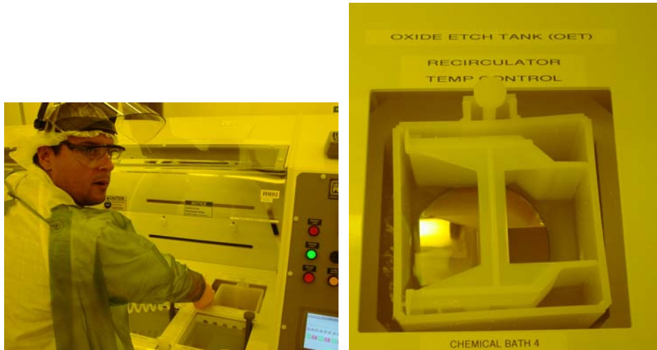
Figure 6. Filling the tank with DI water from spray gun (left) and 6 inch wafers immersed in tank insert (right).
