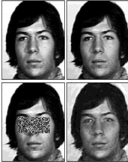
FIG. 3. — Illustration of a content addressable memory for faces. The left panels are the stimuli given as keys to the memory. The right panels are the responses of the memory. The memory is able to reconstruct, reasonably well, a face from an incomplete input (bottom panels). The memory was trained with 160 Caucasian faces (80 males and 80 females), using a Widrow-Hoff learning rule.
