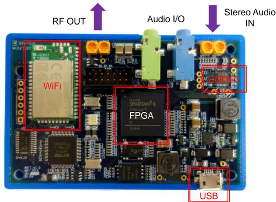
The platform consists of a smart-phone/tablet for implementing and evaluating novel sound processing algorithms and a custom-developed interface board to stimulate Cochlear Corporation's CI24 implants. The interface board houses a high quality stereo audio codec, an FPGA, a Wi-Fi module, and a set of input/output ports for connection with clinical Behind-the-Ear (BTE) microphone units, and Freedom headpiece coils
