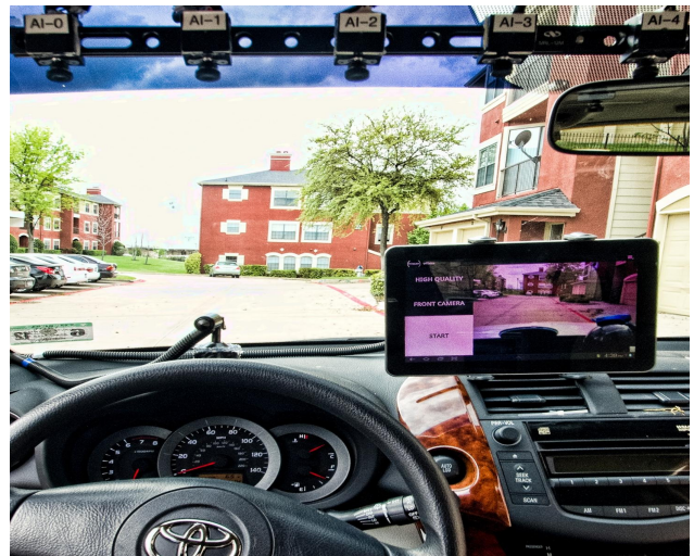
Fig. 2. Inside of the UTDrive instrumented vehicle along with the portable device mounted on the windshield.
