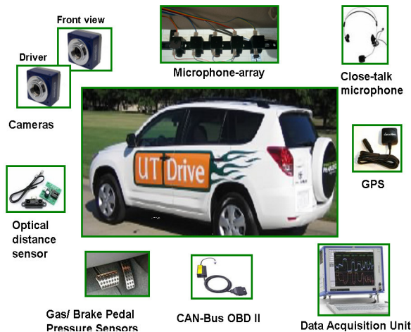
Fig. 1. UTDrive instrumented vehicle with available sensors.
