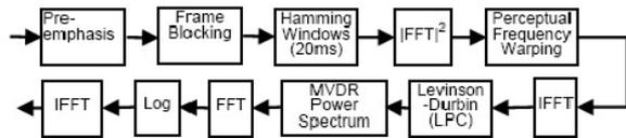
Figure 2: Block diagram to extract PMVDR features.
