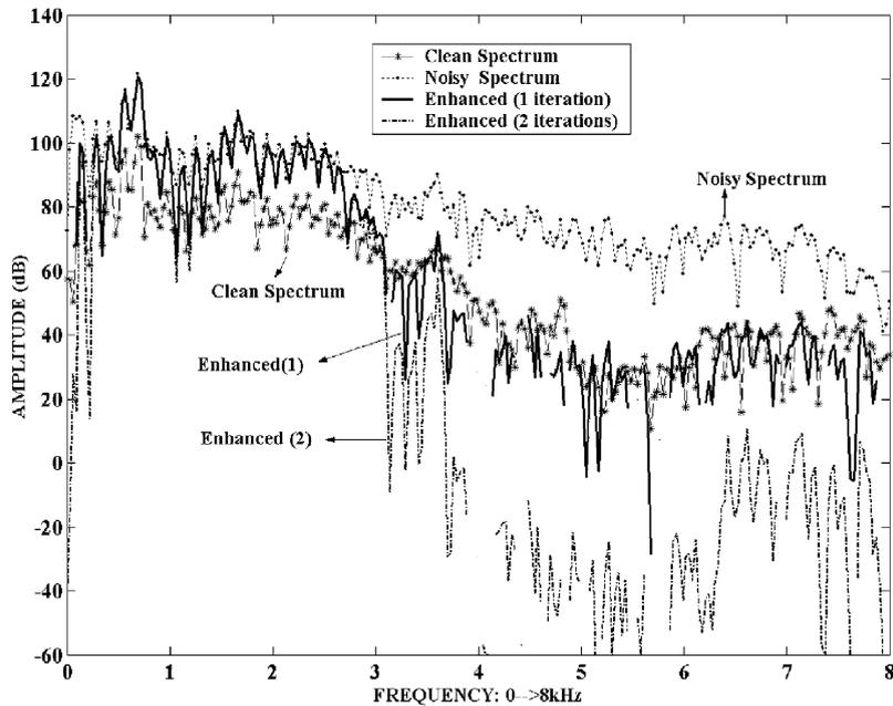
**Spectra for /A/: obtained at 16 kHz sampling rate**
