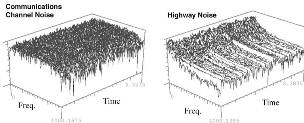
Fig. 2. Time-frequency spectra of the communication channel noise and of the highway noise.
