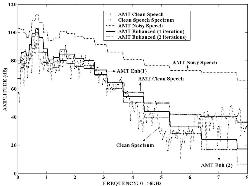
**AMT for /A/: obtained at 16 kHz sampling rate**
