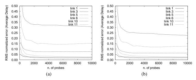
Figure 13: ACCURACY OF INFERENCE: AVERAGE DELAY. Left: d = 1ms. Right: d = 0.1ms. The graphs show the normalized Root Mean Square error between the estimated and sample average delay over 100 simulations.
