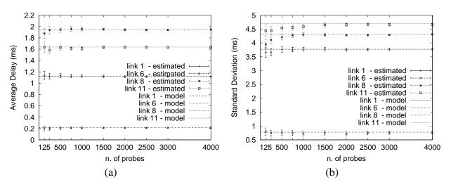
Figure 9: Model Simulation: Topology of Figure 8. Estimated versus Theoretical Delay Average and Standard Deviation with 95% confidence interval computed over 100 model simulations.
