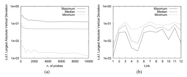
Figure 16: TCP/UDP SIMULATION: TOPOLOGY OF FIGURE 8. ACCURACY OF THE ESTI-MATED DISTRIBUTION. LARGEST VERTICAL ABSOLUTE DEVIATION BETWEEN ESTIMATED AND THEORETICAL C.D.F. Minimum, median and the maximum largest absolute deviation in 100 simulations computed over all links as function of n (a) and link by link for n = 10000 (b).
