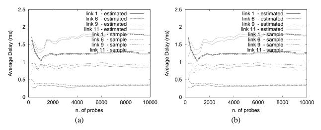
Figure 11: CONVERGENCE OF INFERRED VERSUS SAMPLE AVERAGE LINK DELAY IN TCP/UDP SIMULATIONS. (a): bin-size d = 1ms. (b): bin size d = 0.1ms. The graphs shows how the inferred values closely track the sample average delays.
