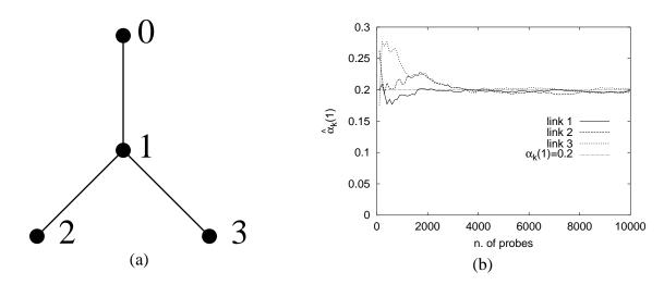
Figure 6: TWO RECEIVERS TREE. (a): Simulation topology. (b): Convergence of  $\hat{\alpha}_k(1)$  to  $\alpha_k(1)$ .  $\alpha_k(0) = 0.79, \alpha_k(1) = 0.2$  and  $\alpha_k(\infty) = 0.01$  for all links.
