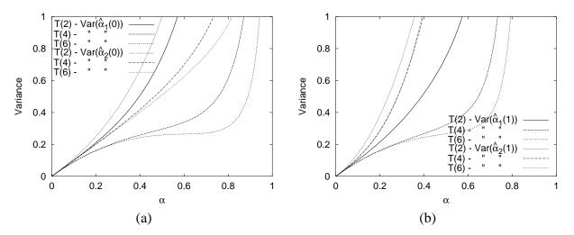
Figure 4: ASYMPTOTIC ESTIMATOR VARIANCE AND BRANCHING RATIO. Binary tree with depth 2 and 2, 4 or 6 receivers. Left: Variance of  $\hat{\alpha}_k(0)$  (a) and  $\hat{\alpha}_k(1)$  (b) for link 1 (common link) and 2 (generic receiver).
