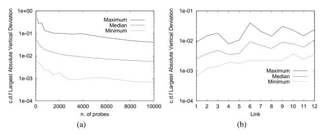
Figure 10: MODEL SIMULATION: TOPOLOGY OF FIGURE 8. ACCURACY OF THE ESTIMATED DISTRIBUTION. LARGEST VERTICAL ABSOLUTE DEVIATION BETWEEN ESTIMATED AND SAMPLE C.D.F. Minimum, median and the maximum largest absolute deviation in 100 simulations computed over all links as function of n (a) and link by link for n = 10000 (b).
