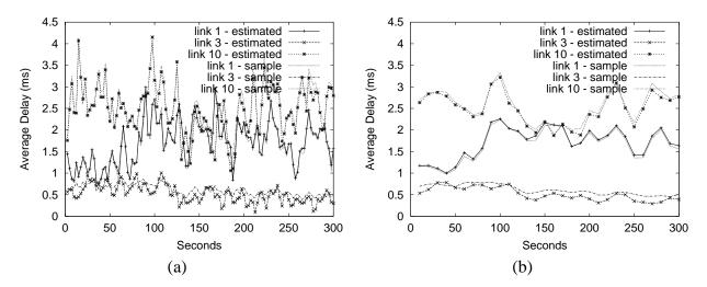
Figure 12: DYNAMIC ACCURACY OF INFERENCE. Sample and Inferred average delay on links 1, 3 and 10 of the multicast tree in Figure 8. (a): 5 seconds window. (b): 20 seconds windows. Background traffic has random start stop times.
