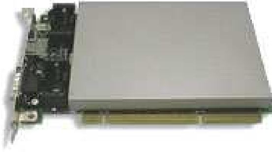
Figure 2.1. IBM 4764 PCI-X Cryptographic Coprocessor
