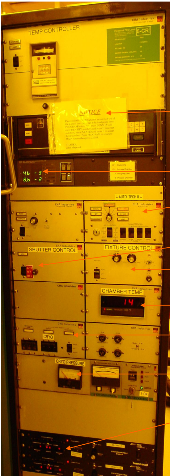
Figure 1. CHA-50 e-Gun Metal Evaporator control rack identifying important controls.
