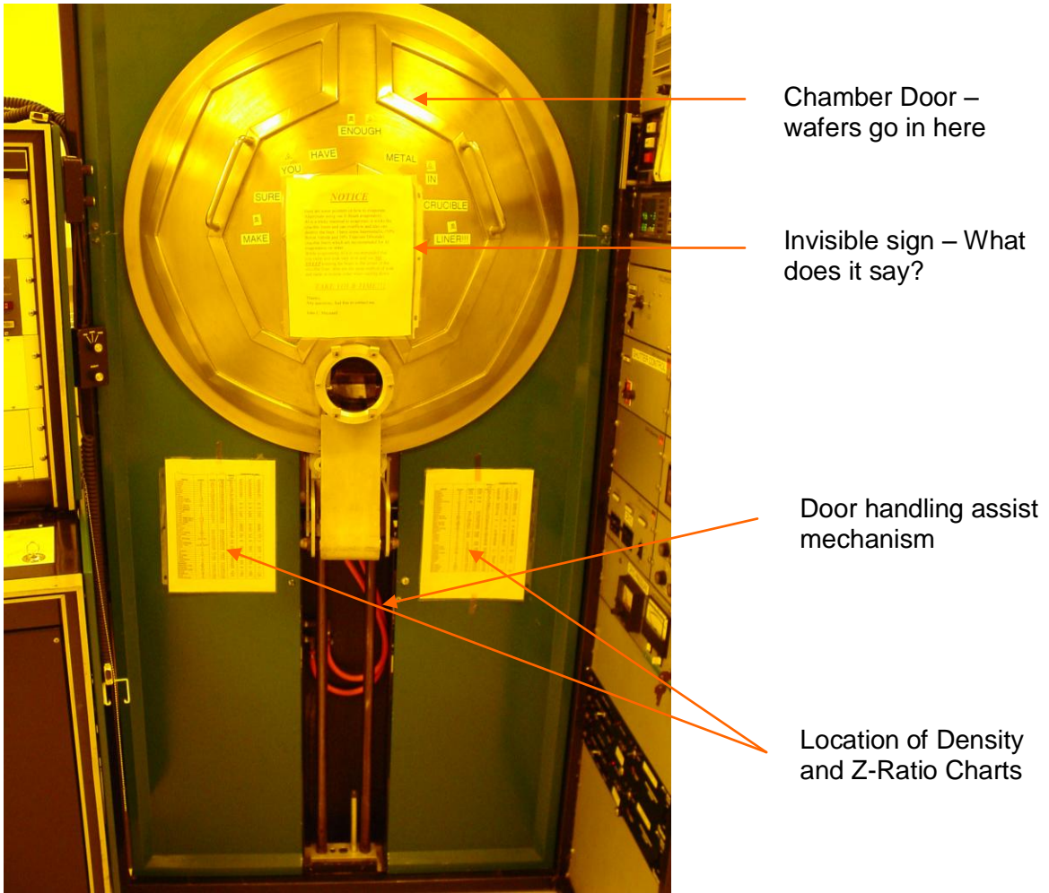
Figure 2. Evaporator Vacuum chamber door with visual port window.
