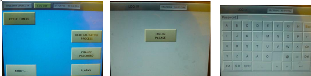
Figure B1. Sequence of screens to enable login. Select Neutralization: Resulting the screen:
