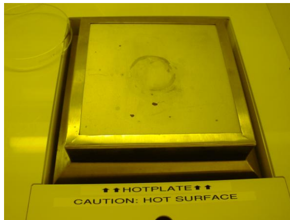
Figure 5. Hotplate showing splash skirt and cover for hotplate control knobs.
