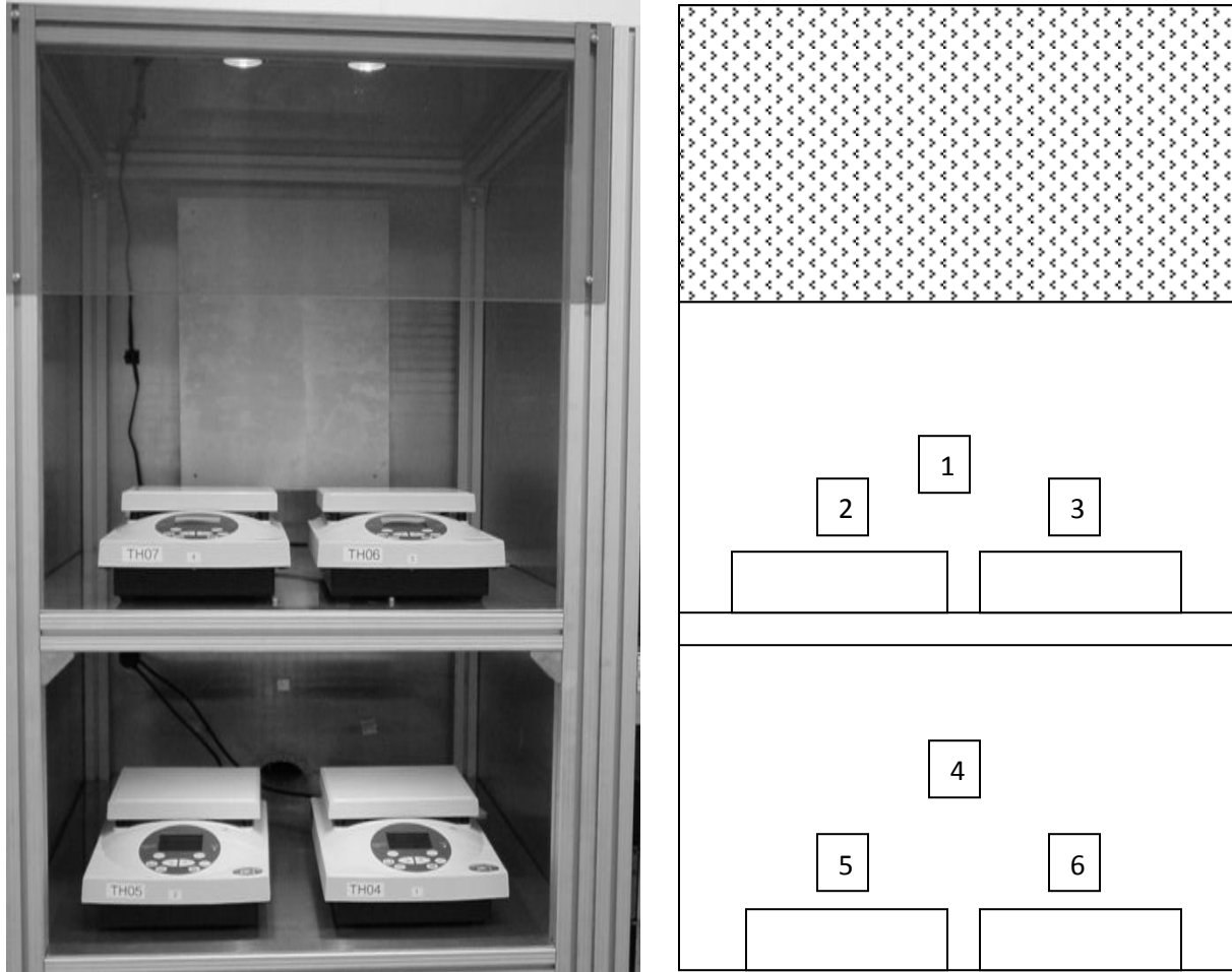
Figure 7. Hotplate exhausted enclosure. Photo on left and schematic on right show the locations of airflow measurements. Boxed 1 and 4 denote the measurement location for the front face airflow just behind the center of the front plane of the enclosure opening. Boxed numbers 2, 3, 4, and 5 represent the airflow about 2 inches above the center of each corresponding hotplate.
