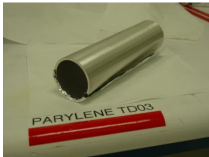
Figure 7. Curl a patch of Al foil around the former cylinder with the bright side against the former tube.
