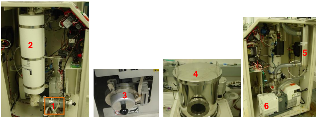
Figure 2. Elements of the Parylene Deposition vacuum system: 1) Vaporizer, 2) Pyrolizer Furnace, 3) Vaporizer Door, 4) Deposition chamber, 5) Cold Trap, 6) Vacuum Pump.
