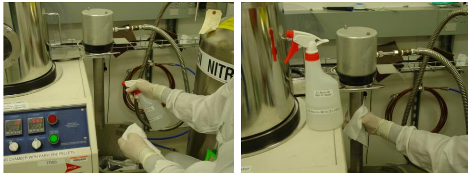
Figure 6. Spraying cold trap with Micro 90 2% DI H 2 O and wiping excess liquid off to reduce future Parylene adhesion for ease in cleanup.
