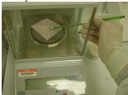
Figure 8. Weigh out the desired mass of Parylene Dimer onto a weighing paper.
