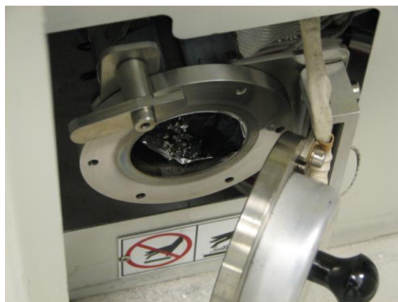
Figure 11. Vaporizer door open for Parylene Dimer insertion.
