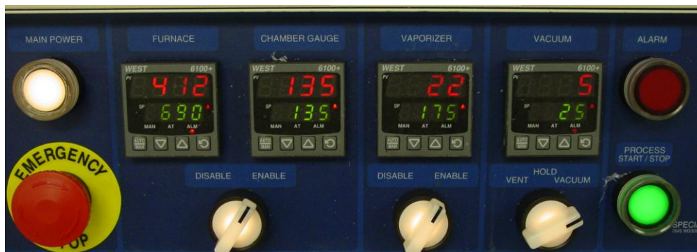
Figure 9. Front panel switches and buttons and process controller readouts. Red numbers (top) are actual readings; Green numbers (bottom) are set point values.
