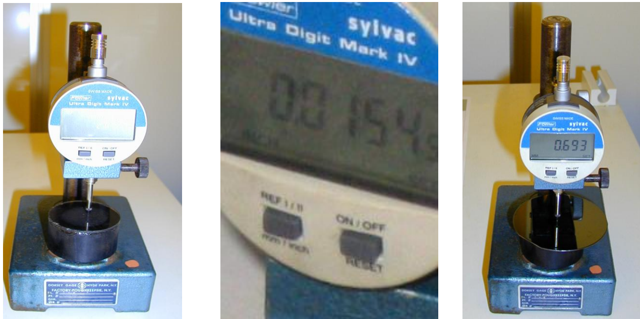
Figure 6: Ultra Mark IV (micrometer) Used to measure wafer thickness. Easy to read liquid crystal display face. Readings can be taken in inches or millimeters.
