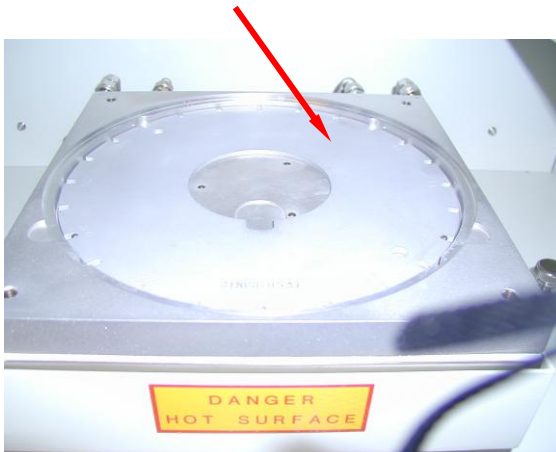
Figure 3a: Ring Locator, used to position the wafer. Notched edges indicate angle of rotation – used for creating 3-D deflection graphs.
