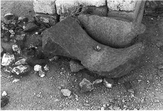
Fig. 17. Concave shaped Ptolemaic gold mill with a two handled mill stone, with a two handled grinding stone, together producing a swinging milling technique and thereby increasing the fineness of the quartz ore powder fraction. Gidami gold mining site, Eastern Desert, Egypt.
