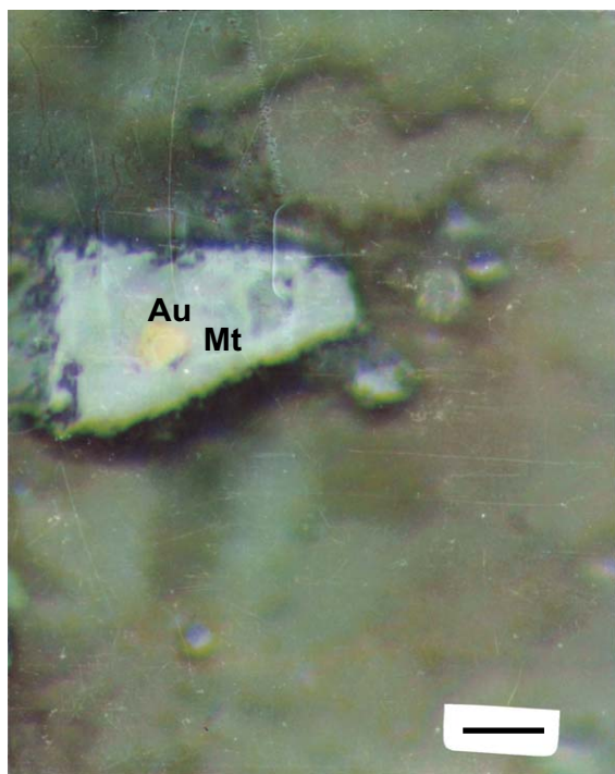
Fig. 21. Photomicrograph showing gold speck (Au) hosted in magnetite (Mt) host, Um Monqul gold prospect, Eastern Desert, Egypt. Reflected light, bar length represents 0.05 mm (from Botros and Wetait, 1997).
