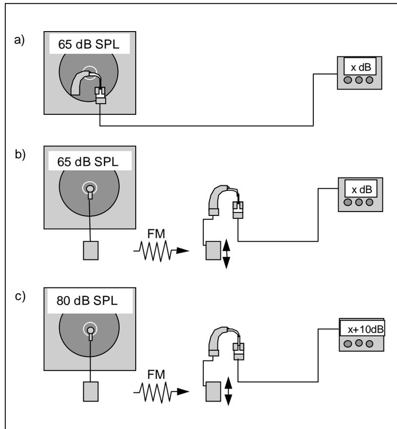
Figure 2. A suggested procedure for adjusting FM gain so as to preserve a 10 dB FM advantage. a) Using a 1000 Hz tone, measure output for 65 dB SPL input to the local microphone. b) Provide 65 dB SPL input to the remote microphone and adjust FM gain to give the same output (the two channels now have equal gain). c) Increase input to 80 dB SPL. If the output increases by 10 dB, the process is complete. If it does not, increase FM gain to give an FM advantage of between 5 and 7 dB (see text).
