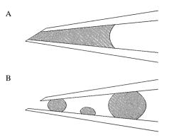
Fig. 4. (A) In a properly silanized micropipette, the liquid membrane solution forms a uniform column with a concave interface against the aqueous filling solution. (B) In a poorly silanized micropipette, the organic membrane solution is easily replaced by water at the hydrophilic glass surface which results in convex interfaces and, often, breaking of the membrane column.
