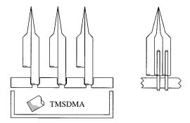
Fig. 6. Holder that allows selective silanization of individual barrels of double or triplebarrelled micropipettes. For details, see text.
