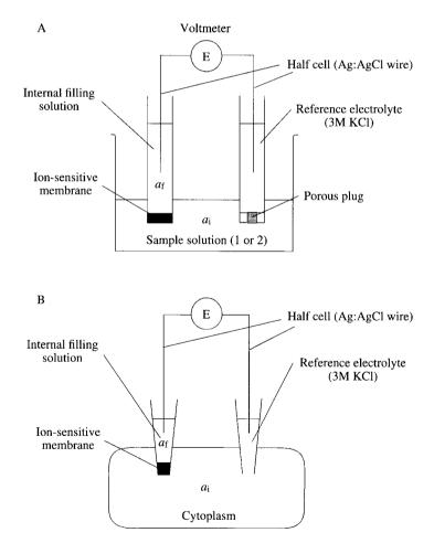
Fig. 2. Experimental set-up for ion-sensitive electrodes. The potential difference E, which exists across a selectively permeable membrane is measured by a voltmeter.  $a_f$  and  $a_i$  denote the activity of the permeant ion in the filling solution and in the sample solution respectively. For details, see text.
