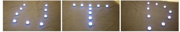
Fig. 1. Proposed formation control strategy implemented on our distributed wheeled mobile robotic platform to form the letters UTD.
