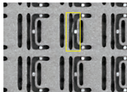
Figure 4: Top down SEM image of the pattern related bridging defect discussed in case study II
