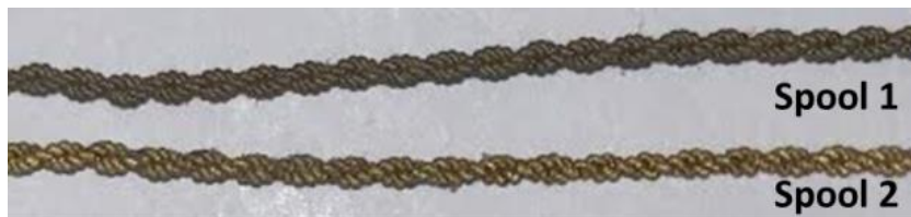
Figure 4: Samples of fabricated 2-ply muscles from spool 1 and spool 2.
