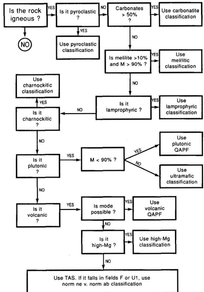
Fig. 8. Simplified flow chart, beginning at the top left, showing the sequence followed by the IUGS scheme for naming an igneous rock using the individual classifications described.
