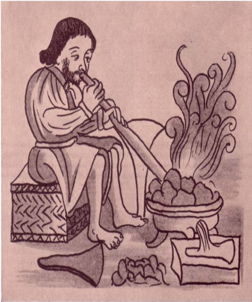
AXE-BLADE CASTING as practiced in Mexico is depicted in Bernardino de Sahagún's study of pre-Columbian technology. Copper was brought to melting temperature with a blowpipe; the molten metal ran out of a furnace tap into a stone mold. On the ground is a finished axe blank; this will be given its final form by hammering (see illustration below).
