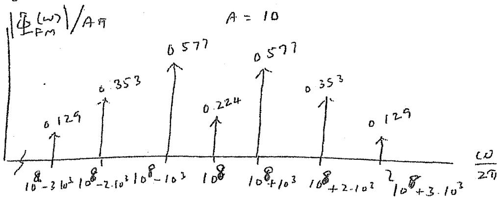
A signal  $m(t)$  frequency modulates a 100 kHz carrier to produce the following narrowband FM signal:
