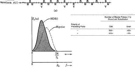
000V and B00V, where B=1 conforms to the bipolar rule and V=1 violates the bipolar rule. The choice of sequence 000V or B00V is made in such a way that consecutive V pulses alternate signs in order to maintain the dc null in PSD.
