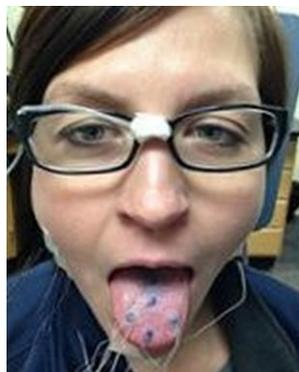
Figure 2: Positions of tongue sensors and head sensor (on glasses).
